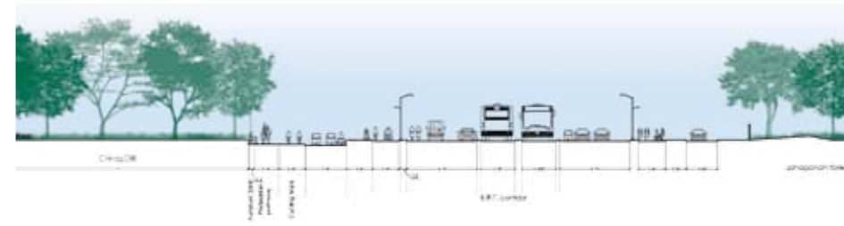
Typical section along Linkage I (Along forest) (Section along Ring Road at Jahanpanah Forest)
