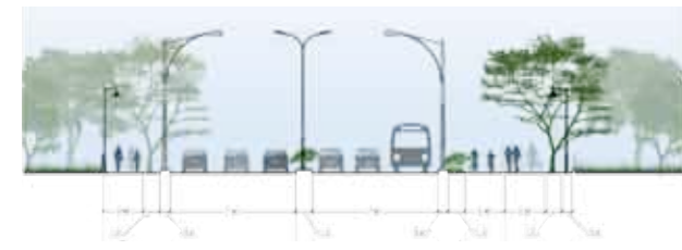
CC' –Typical Section Across Linkage 2 (Arterial Road)
